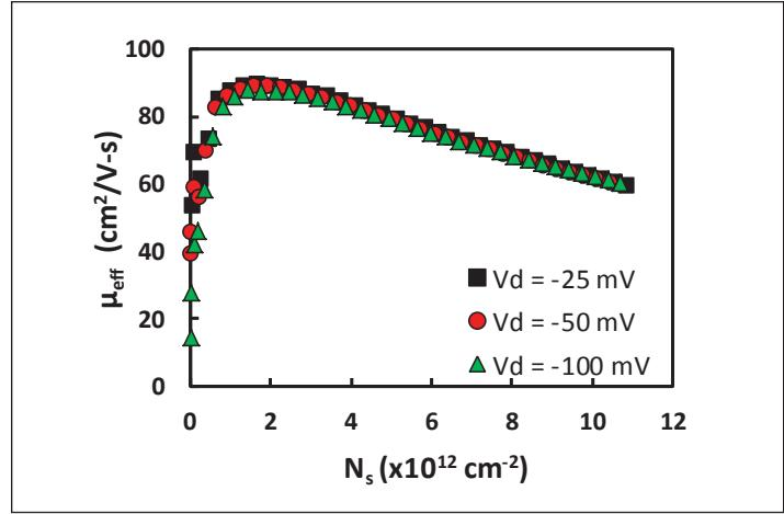
Figure 7. The effective channel mobility,  $\mu_{eff}$ , extracted under three different  $V_d$  by using UFSP technique.
