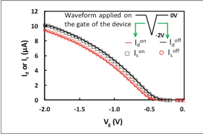
Figure 5. Four currents measured from source and drain corresponding to the off-to-on and on-to-off  $V_g$  sweep. Schematic  $V_g$  waveform is shown in inset.
