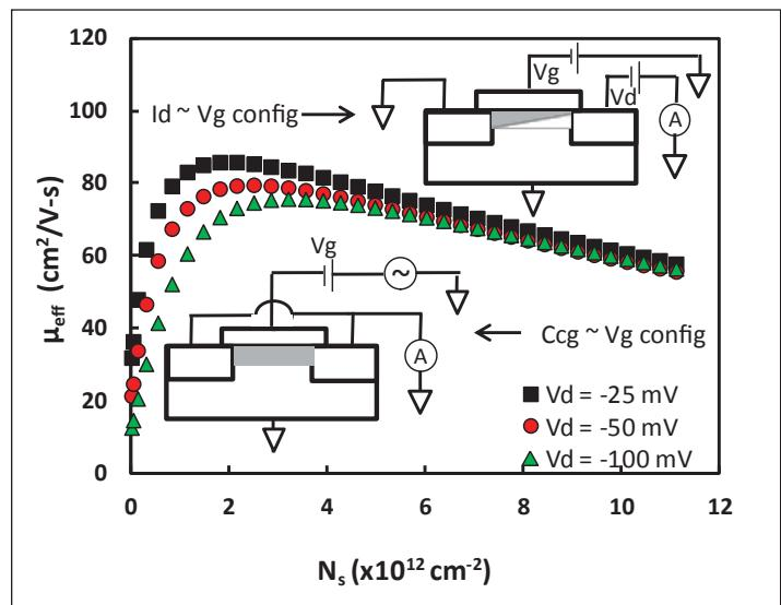
Figure 2. Effective channel mobility measured by conventional technique.  $I_{\text{ch}}$  was measured under various non-zero drain biases,  $V_{\text{DS}}$ , but  $Q_i$  was measured under  $V_d = 0$ . The extracted mobility clearly reduces for higher  $|V_d|$ . Insets illustrate the carrier distribution in the channel.
