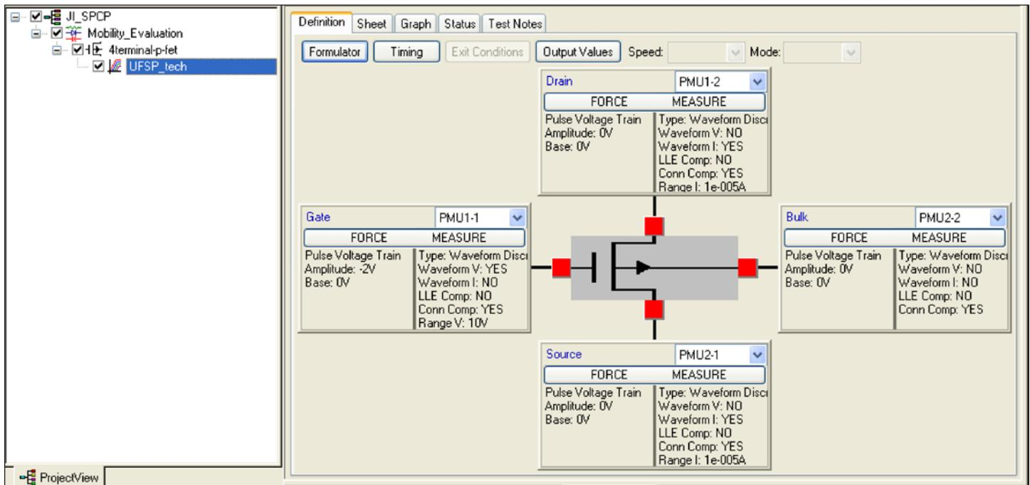
Figure 12. Example project in KTEI software for UFSP measurement. Each of the four terminals of the device is connected to one channel of PMU respectively.
