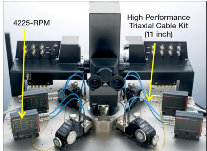
**Figure 10.** Photo of the UFSP technique setup using Keithley instruments.
