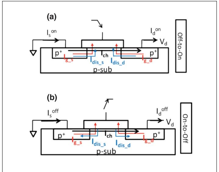
**Figure 4. Schematic diagram of current flow during the transient measurement.**
