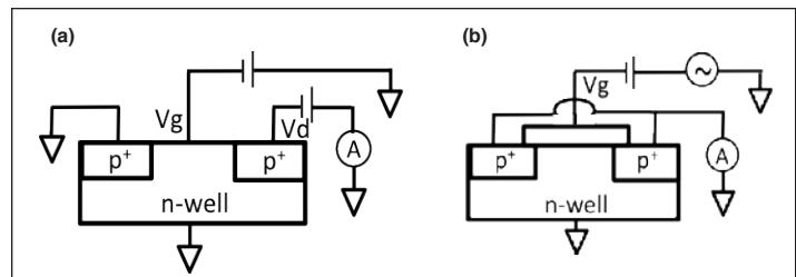
Figure 1. Configuration for (a) conduction current measurement and (b) gate-to-channel capacitance,  $C_{\text{gc}}$ , measurement.
