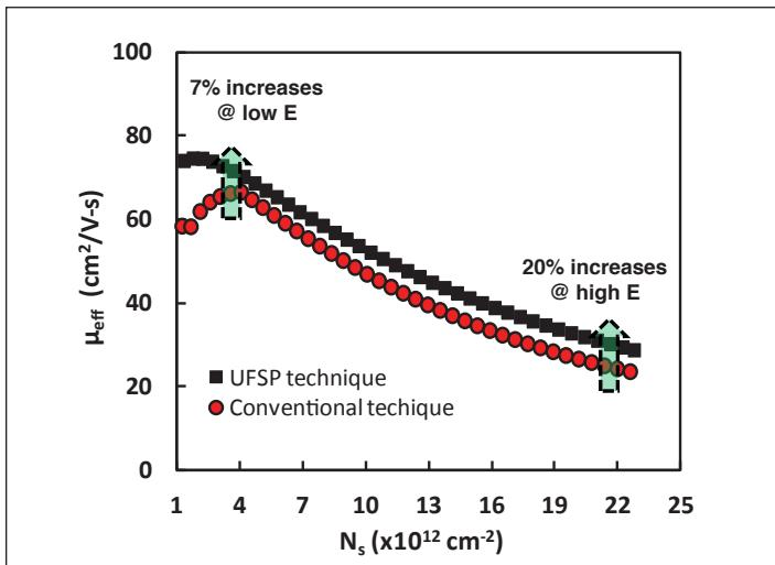
**Figure 9.** A comparison of mobility extracted by UFSP and conventional technique for a device with  $\text{HfO}_2/\text{SiON}$  dielectric of considerable fast trapping.
